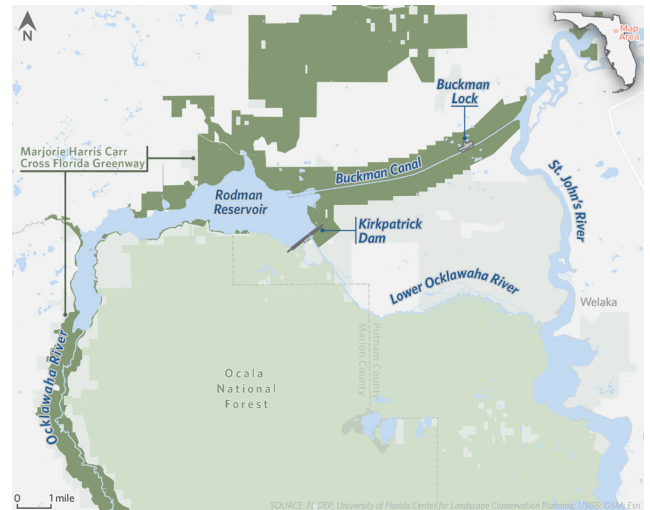
Figure 2. The Kirkpatrick Dam is a 22-foot-high, 6,800-foot-long earthen structure with four gates and a concrete spillway (Shuman 1995).
